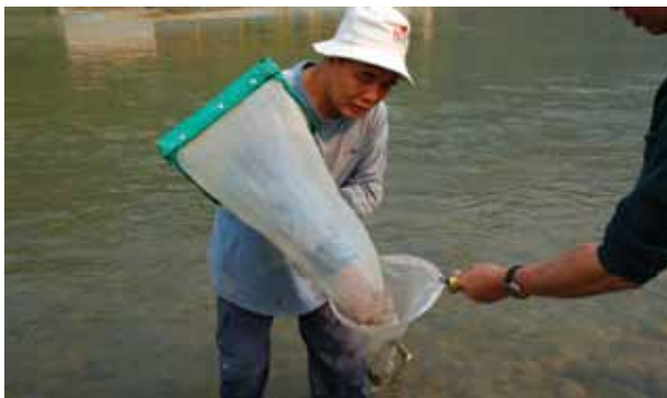
Step 2. The D-frame net is then inverted and its contents emptied into a hand net or sieve.
