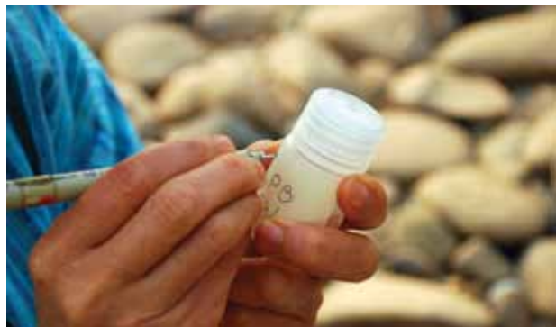
Step 7. The sample jar is labelled with the site name, site code, date, and sample replicate number.
