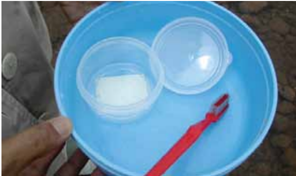
Step 3. Toothbrushes, plastic bowl, plastic containers with sealable lids, Lugol's Solution, labels and a marker pen used for sampling.
