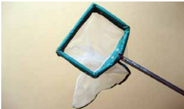
A D-frame net with 30cm x 20cm opening and mesh size of 475µm is used for sampling.
