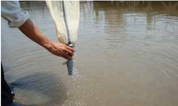
Step 4. Rinse the bottom of the net to result in a water volume of about 150mL.
