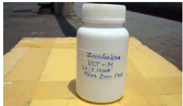
Step 7. Label the sample jar (site name, site code, date, location in the river).
