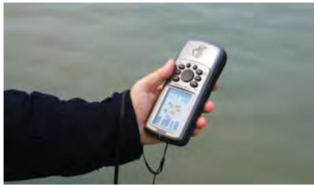
Altitude and coordinates of the sampling site are measured using a GPS device
