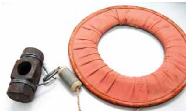
Water depth determined by dropping a weighted rope directly to the river bottom
