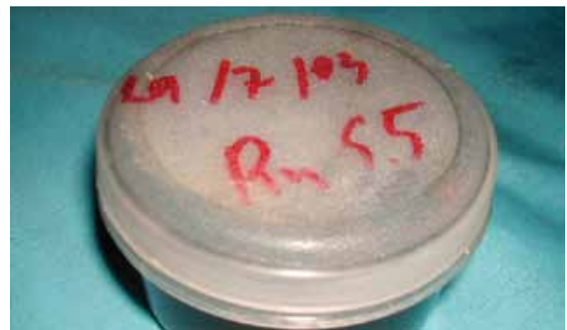
Step 8. The label includes the site name, the site code, the date, and the replicate number, written on the plastic container.
