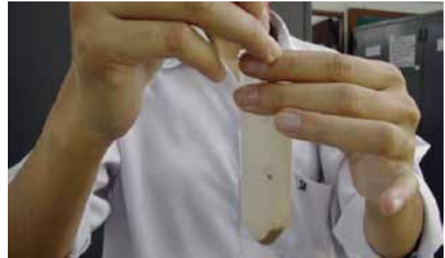
Step 2. The diatom cells are the brown layer between the supernatant and solid particles.
