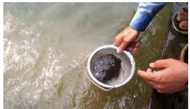
Step 5. Remove some of the sample and place it in a smaller-sized sieve with a 0.3mm mesh for further washing.
