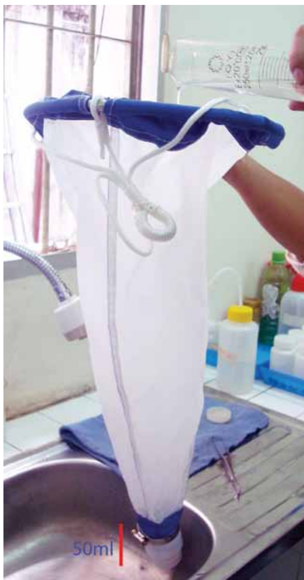
Step 3. Filter the sample through a net with a mesh size of 10\mu\text{m} , to result in a total volume of 50mL.
