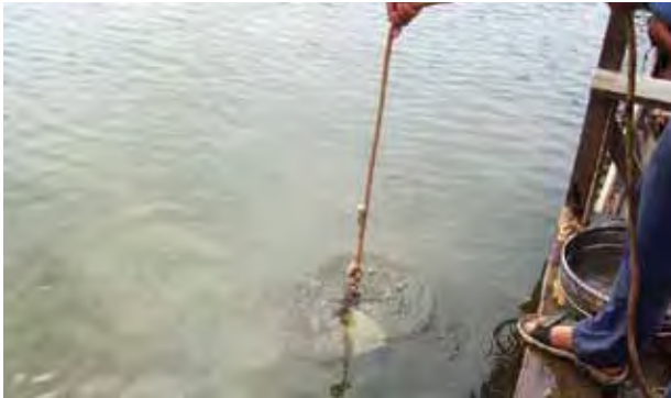
Step 2. Lower the grab into the water, making sure that it catches on the river bottom.
