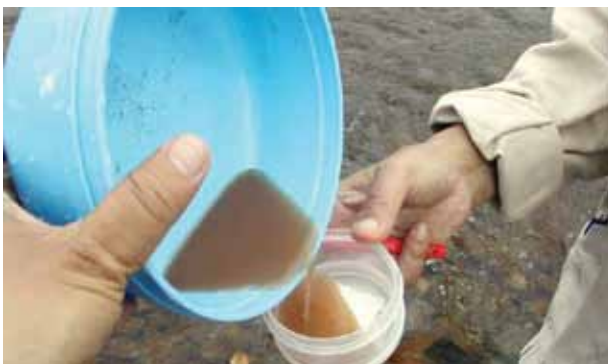
Step 7. Each sample is poured into a plastic bowl and then into a plastic container.
