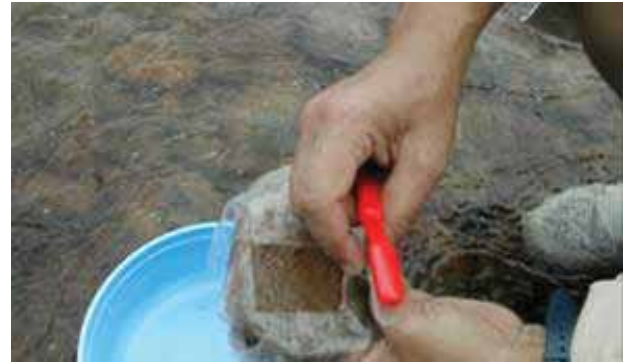
Step 4. A plastic sheet with a 10 cm 2 cut-out is placed on the upper surface of the selected stone.
