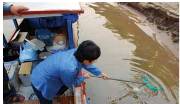
Step 1b. In deep water, the collector stands on a boat about 1 - 1.5 m from the water's edge and sweeps the net towards the bank, near the substrate surface.
