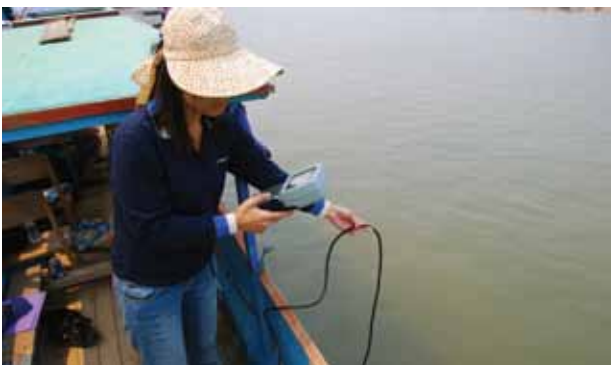
Temperature, DO, pH, EC are recorded using an electrical metre
