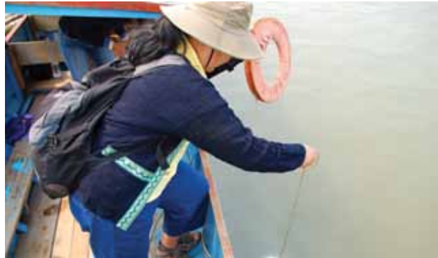
Light penetration is recorded by slowly lowering the Secchi disk into the water until it just disappears
