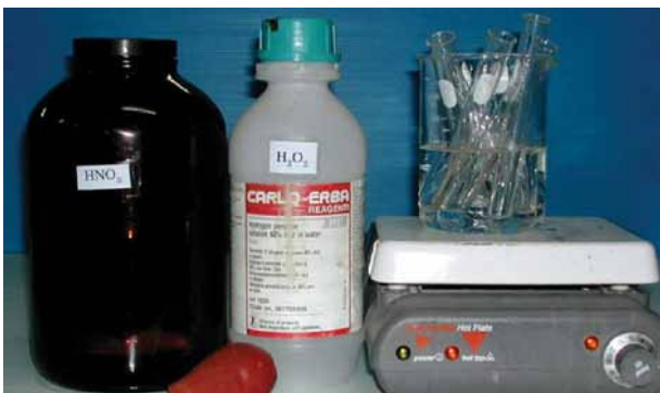
Step 3. Strong acid ( H_2SO_4 , HCl or HNO_3 ) is added and the tubes are heated ( 70 - 80^\circ C ) for 30 - 45 minutes.
