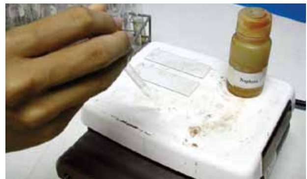
Step 6. A drop of a mounting agent is added, followed by the addition of a cover slip, to make a permanent slide.
