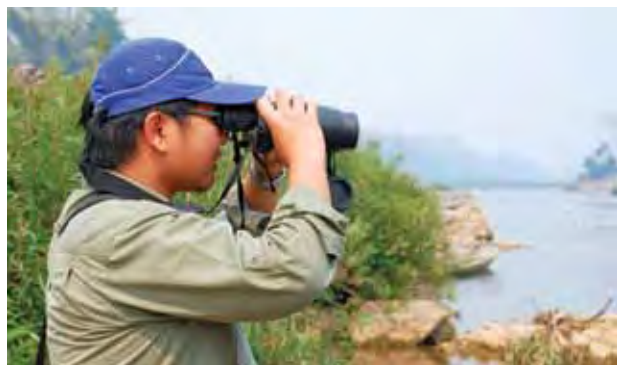
River width is measured using a laser rangefinder
