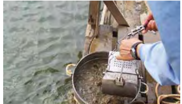
Step 3. Release the contents from the grab into a stack of sieves with the largest mesh size on the top, and the finest at the bottom.
