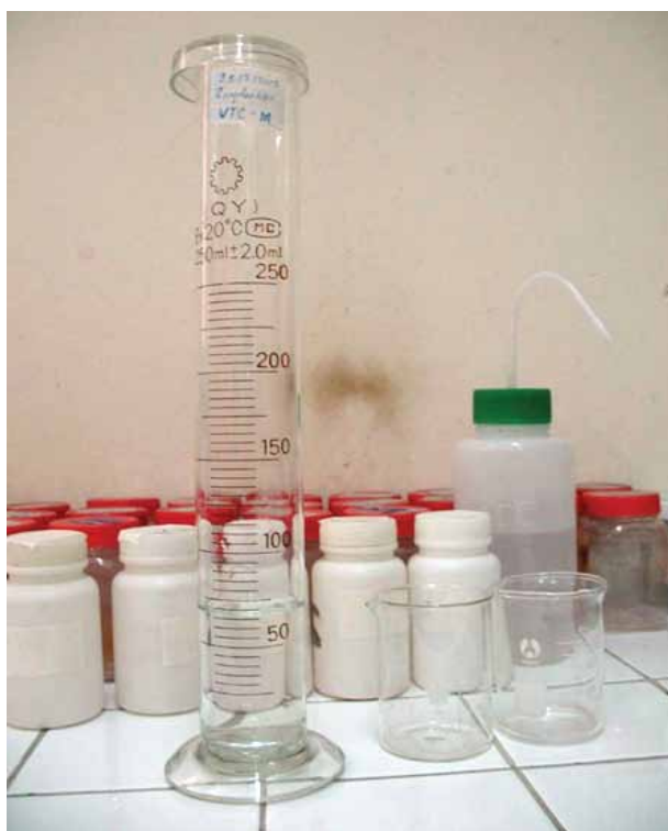
Step 2. Allow the sample to settle in a cylinder for about 1 hour.
