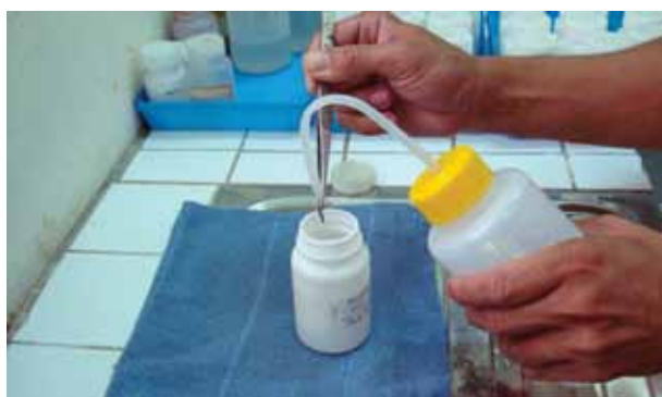
Step 1. Use forceps to remove large debris from sample.
