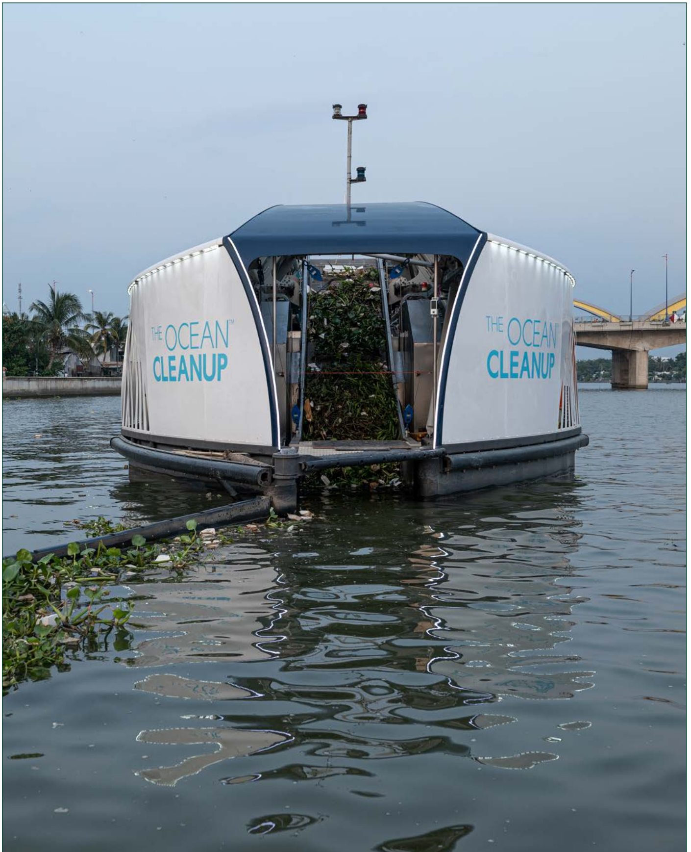
The floating barrier (left) of "Interceptor 003" leverages tides and currents in the Mekong Delta to direct plastic and other river detritus to the vessel's conveyor belt. Inside are six 8 m 3 containers. Once full, a barge collects the trash and transfers it to a treatment facility.
