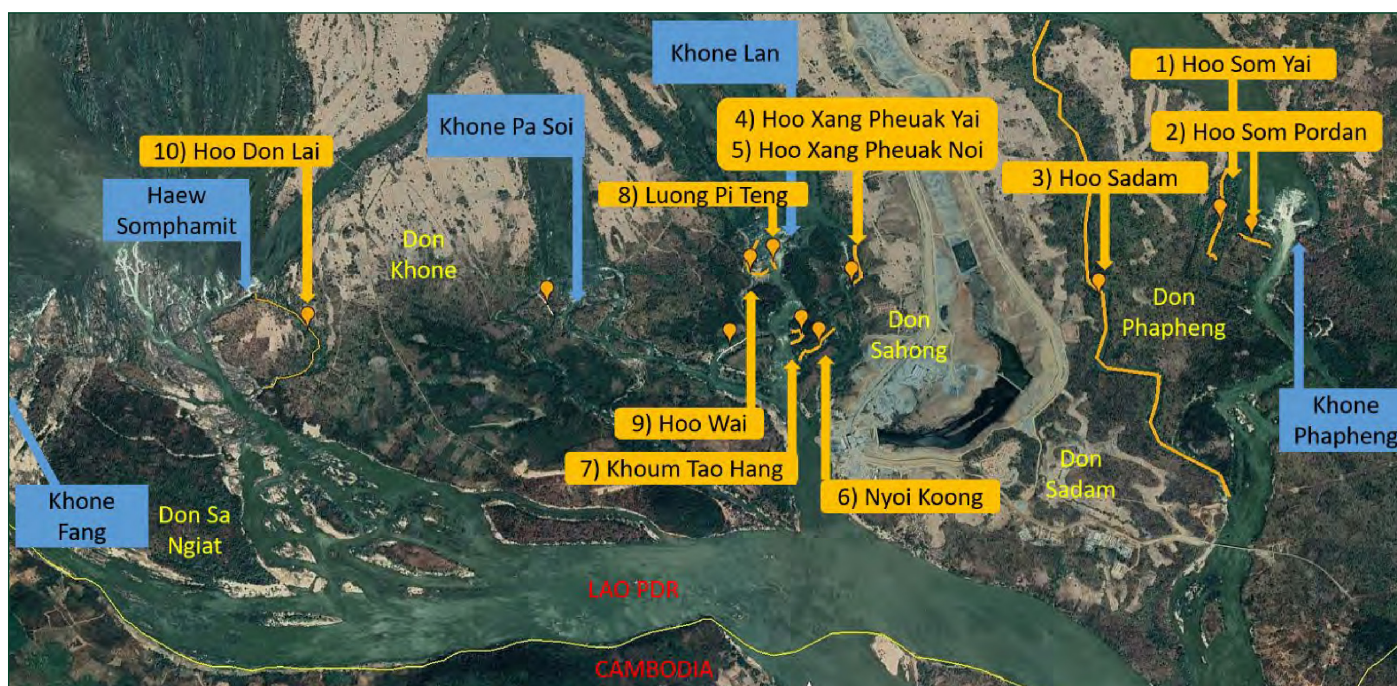
The Khone Falls area on the Mekong River in southern Lao PDR. Major waterfalls are shown in blue and major islands in yellow. Channels improved by Don Sahong Power Co Ltd to encourage fish swimming upstream from Cambodia to complete their migration are shown in orange.
