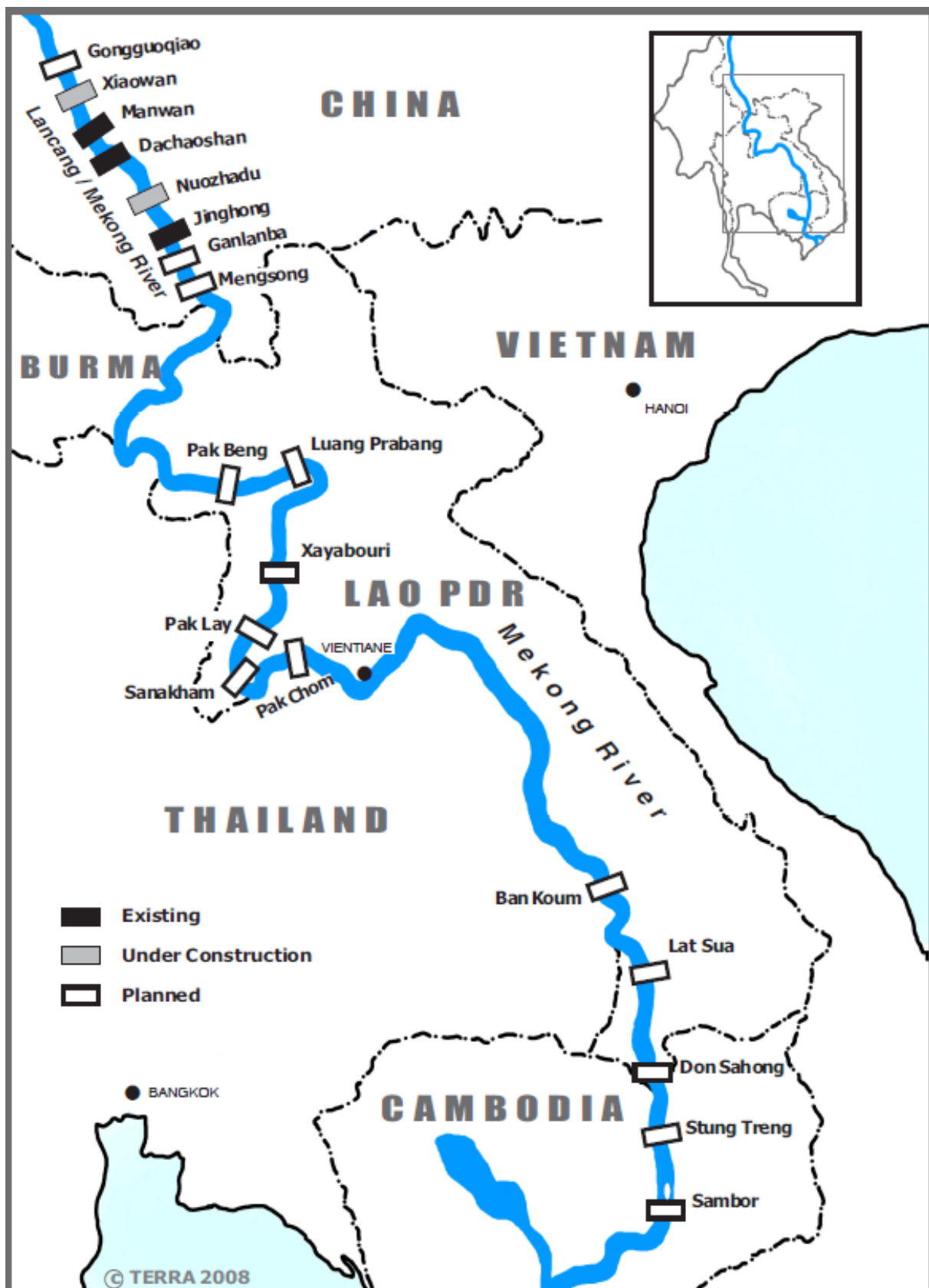
Figure 2. A schematic sketching of the MRB and the main stream hydropower dams that were existing, under construction and planned in the year of 2008. Source: Lee (2008). Courtesy of Terra, reprinted with permission.
