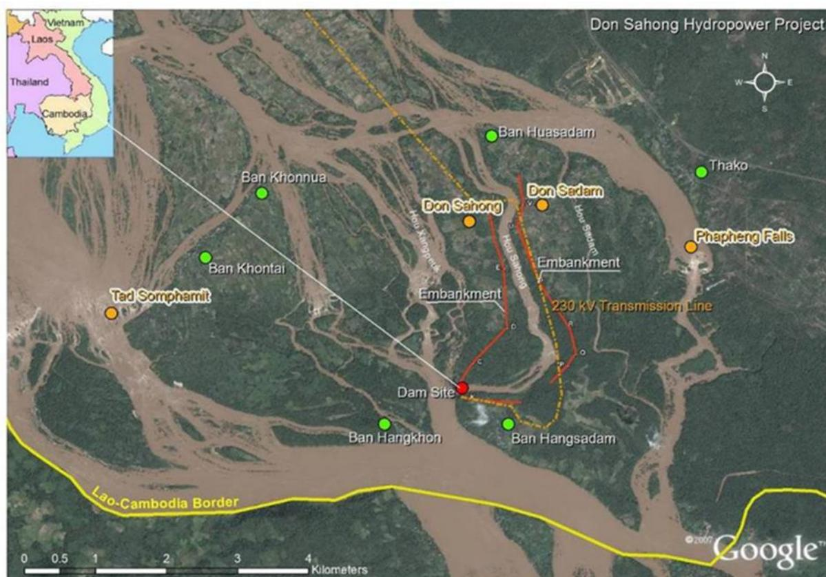
**Figure 1 Locations of DSHPP Barrage Power station and embankment on the Hou Sahong**
