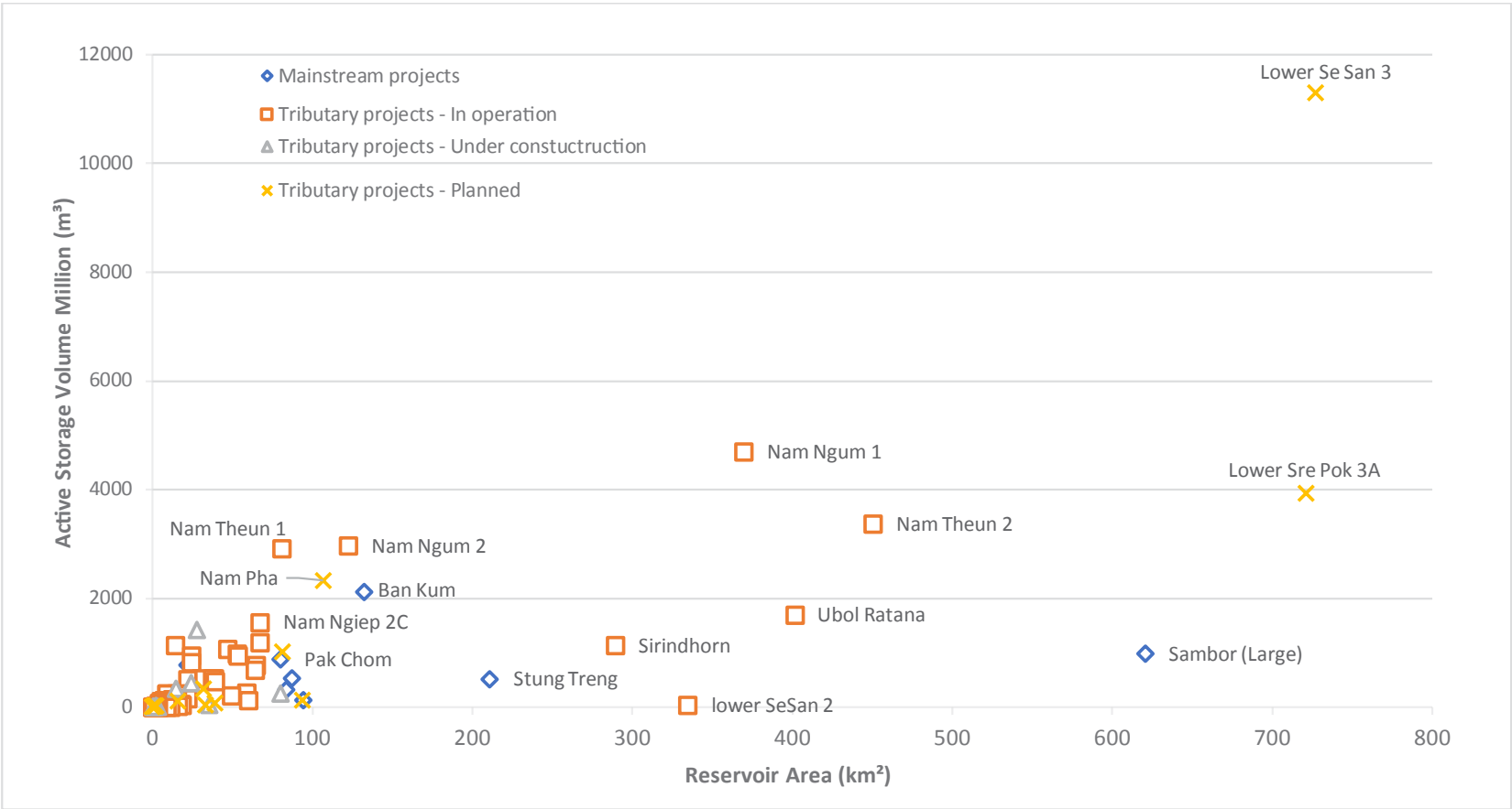
Figure 17. A plot of predicted mean reservoir area (averaged over the year) versus live storage for hydropower projects that are operational and under construction in the LMB
