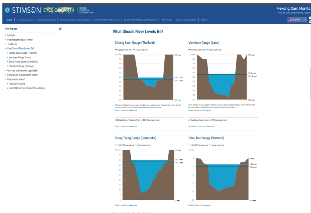
Figure 35. Screenshot of the Mekong Dam Monitor showing the actual and expected water levels at four different river stations (Stimson Center, 2022).
