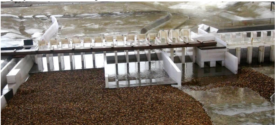
Fig. 2.3.5-1 Downstream in the scour pit ( Q=16700\text{m}^3/\text{s} , ①②③surface bays all with an opening of 8.33m+④⑤⑥⑦⑧surface bays all with an opening of 11m+⑨⑩⑪⑫⑬⑭surface bays all with an opening of 2m)
