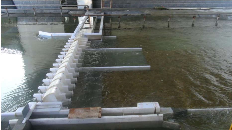
Fig. 2.3.2-2 Operating condition 9 ( Q = 34895 \text{ m}^3/\text{s} , 2 low-level outlets and 14 surface bays fully opened) main energy dissipation area
