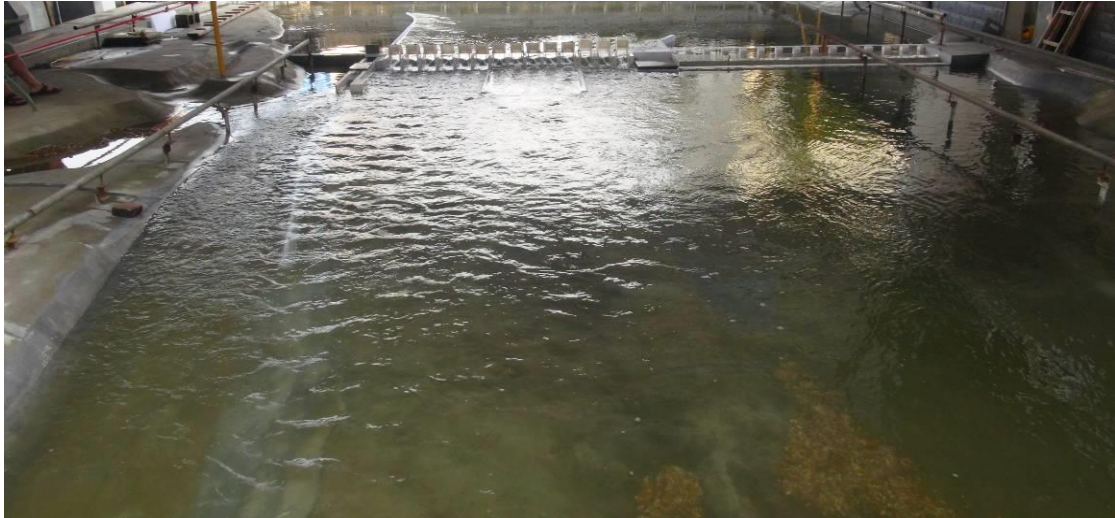
Fig. 2.3.2-3 Operating condition 9 ( Q=34895\text{m}^3/\text{s} , 2 low-level outlets and 14 surface bays fully opened) downstream flow regime
