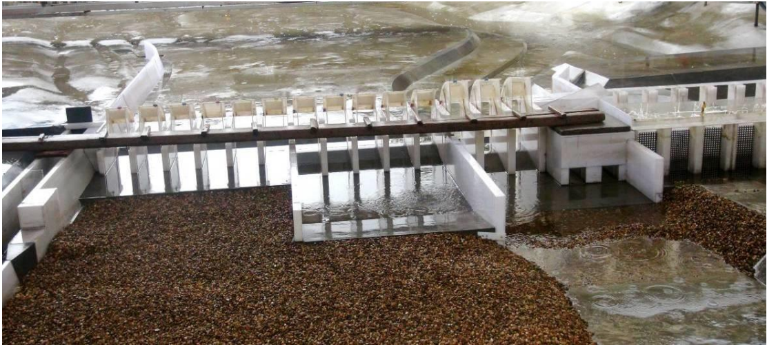
Fig. 2.3.5-3 Downstream in the scour pit (service condition 10, Q=38000\text{m}^3/\text{s} , 2 low-level outlets and 14 surface bays fully opened)
