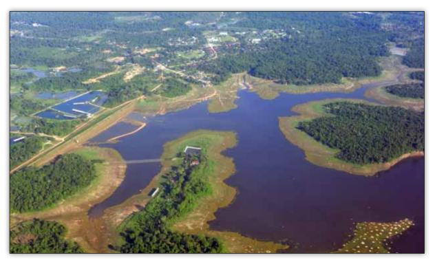
Permanent waterbodies outside the major flood and rainfed zones are mainly reservoirs, like this typical small irrigation reservoir, Nam Houm, in Lao PDR. Fish ponds can be seen downstream of the dam wall on the left.
