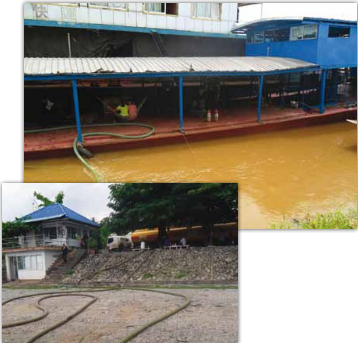
Figure 44: Fuel Transfer from Truck to Vessel at Keawalee Pier
