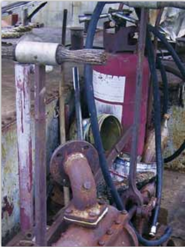
Figure 54: Fire Extinguishers in Poor Condition and Not Readily Accessible
