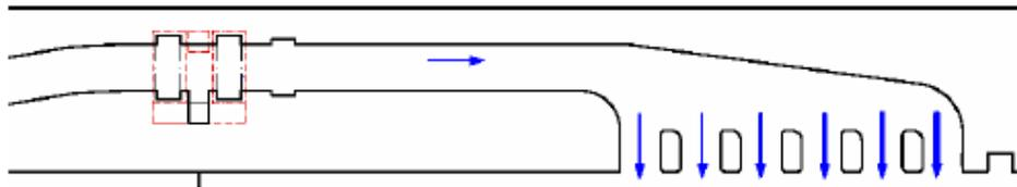
Figure 3: scheme of heterogeneous distribution of flow
