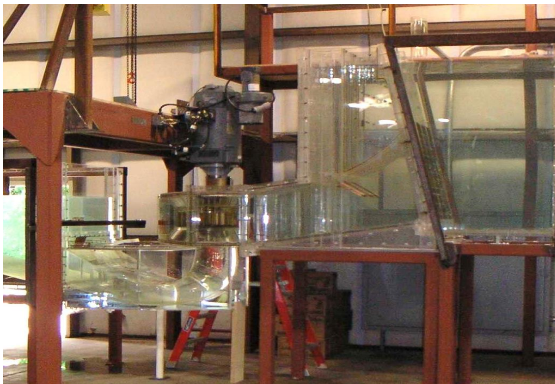
Figure 13: The Ice Harbor turbine 1:25 scale model used to evaluate fish passage conditions
