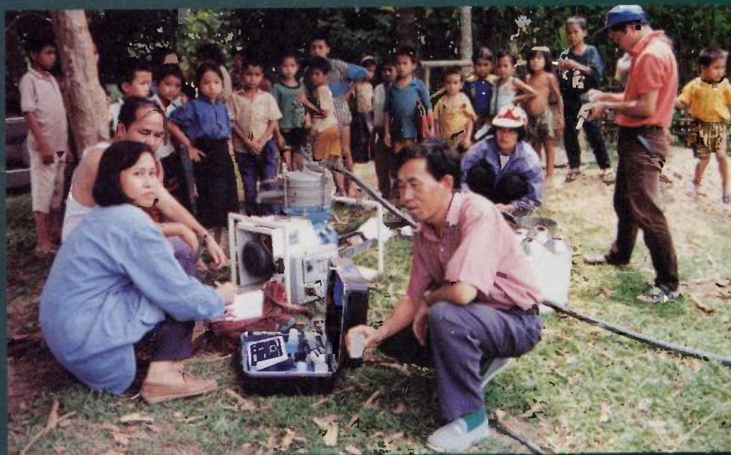
Sampling of suspended sediment, Khammouane Province, the Lao PDR.
