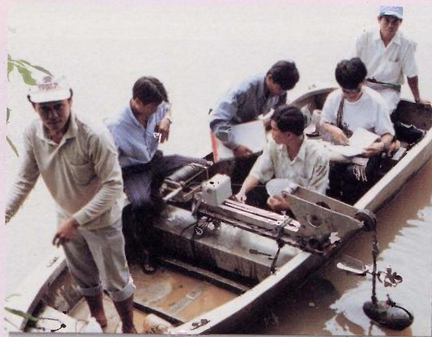
Discharge measurement at Pak Khanhoung, Nam Ngum, the Lao PDR.
