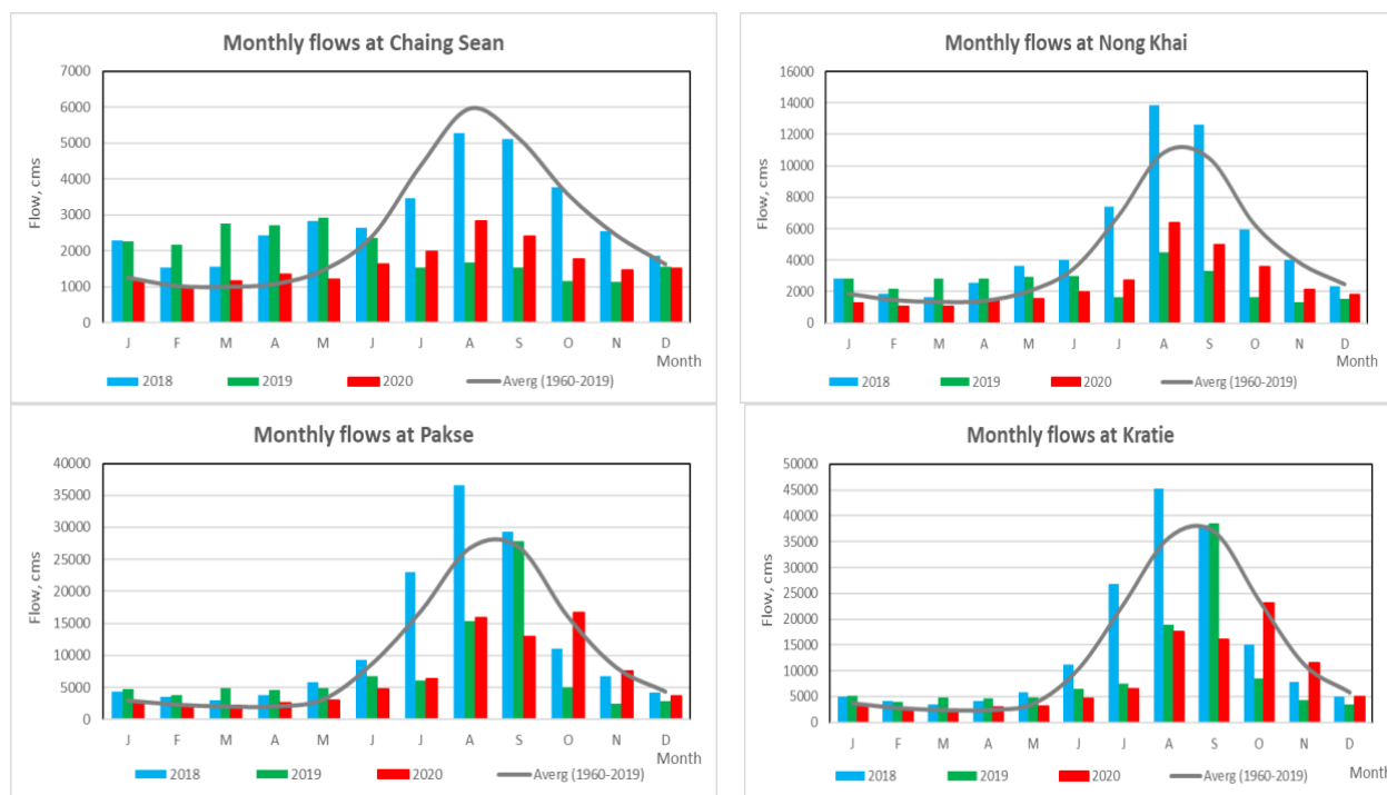
Figure 4. The 2018, 2019 and 2020 rated monthly flows at selected sites on the Mekong mainstream from Chiang Saen to Stung Treng compared to long-term averages.
