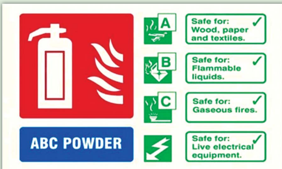
Figure 14: Luminous Sign for Dry Powder Extinguisher
